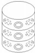
Figure 7 – Shell Buckling
